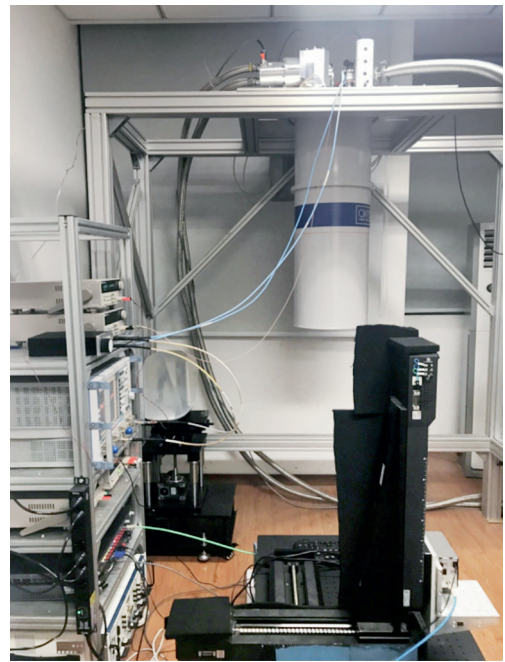
Figure 1. The 32 \times 32 superconducting imaging array system for the 350 \mu\text{m} band.
